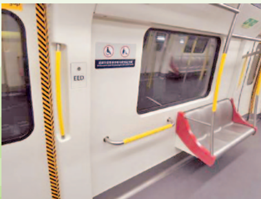
車廂內的多用途空間 Multi-purpose space inside train compartments
